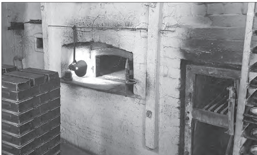
The historic Bodalla Bakery Scotch Oven – fire box at the right and flue to the left.
