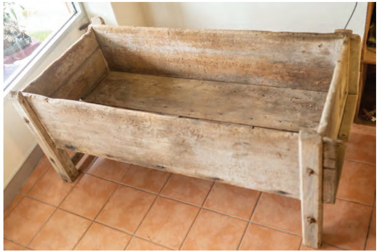
Wooden Cheese-Making Vat. This simple wooden cheese vat, now in the Cobargo Museum, is a historic reminder of the many small-scale dairy operations that were common in the area in the 19th and early 20th centuries. Believed to have been used on a dairy farm in the Cobargo area, this wooden vat enabled cheese to be produced from raw milk without the need for a starter culture - the wood surface providing the required microbial biofilms to transform milk curd into cheese. More details: bit.ly/begahh15 . Image: ‡
