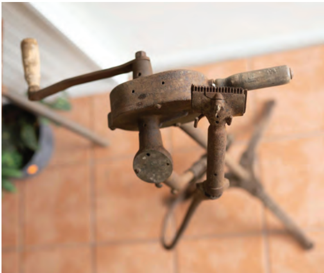
Portable Shearing Plant. An early 20th century R.A. Lister and Company portable shearing device, known to have been used in the Cobargo area, and now in the Cobargo Museum. It would be taken and used anywhere on a property. One person would wind the arm to power the motor, a second person would use the shearing handpiece. More information: bit.ly/begahh14 Image: ‡
