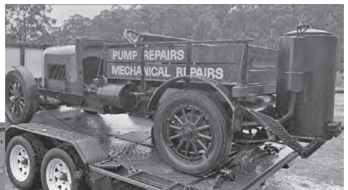
A 1924 Charcoal-burning Dodge Ute, on the way to the Cooma Car Club Museum
